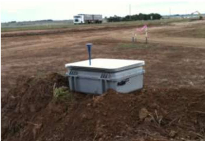
Figure 1. DUSTTRAK™ portable dust monitor. Non-ideal mounting configuration.
